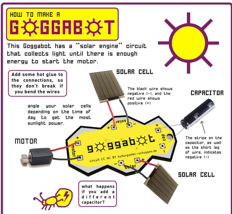
If you have a vibration motor, stick on some brush bristles or thin wire legs with some hot glue. If you have a regular motor, try make a body with wire and/or wheels.
